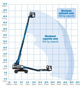
\* The metric equivalent of working height adds 2 m to platform
